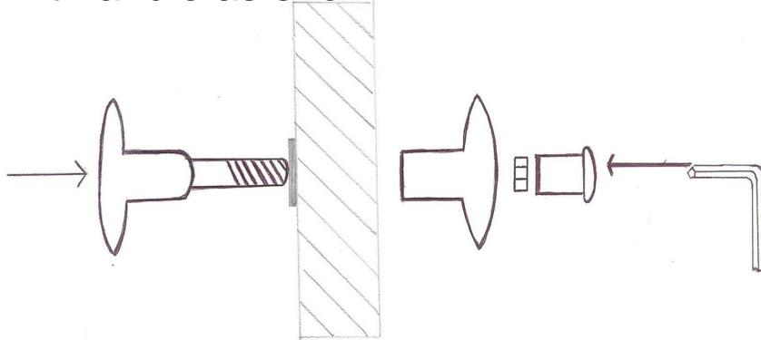
Push the outer handle with the threaded shaft through the outside panel , fit the internal handle nut and moulded fixing with an allen key,check the doors are level and lock correctly , a cause of incorrectly locking doors is if the sides are not plumb if required undo the brackets level the unit and re fix the brackets that hold the sides to the front .
